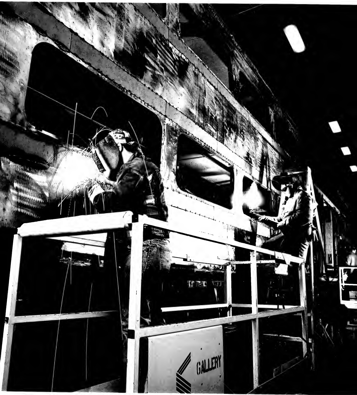
▲ Programming the RTA's $1 billion in bonding authority continued in 1993. Here Metra Electric cars are refurbished at the former Pullman rail car factory on Chicago's South Side.
